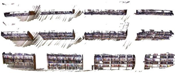
Fig. 5. Rendering of the the points given by frame-to-frame transformation estimates when walking past a series of bookshelves in the KTH library. The data is displayed from three different view points. The bookshelves are lined up in the library and the upper part of the image shows that our method produces results very close to this even using pure dead-reckoning.
