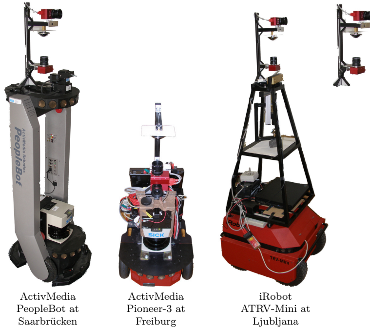
Figure 3: Three different mobile platforms employed for image acquisition at the three labs. The portable socket with the camera setup is shown in the top right corner.
