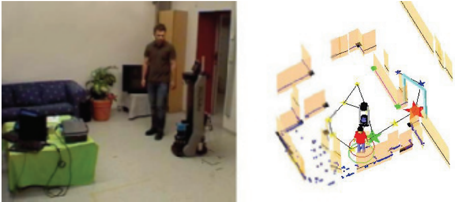
Fig. 10.1. The user shows the Explorer robot where the living room is. The robot's visualization of a similar situation can be seen on the right-hand side.
